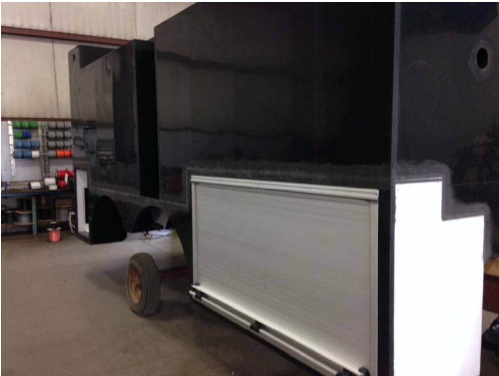
The first compartment door is installed on the body box for the new Solon Tender 1
