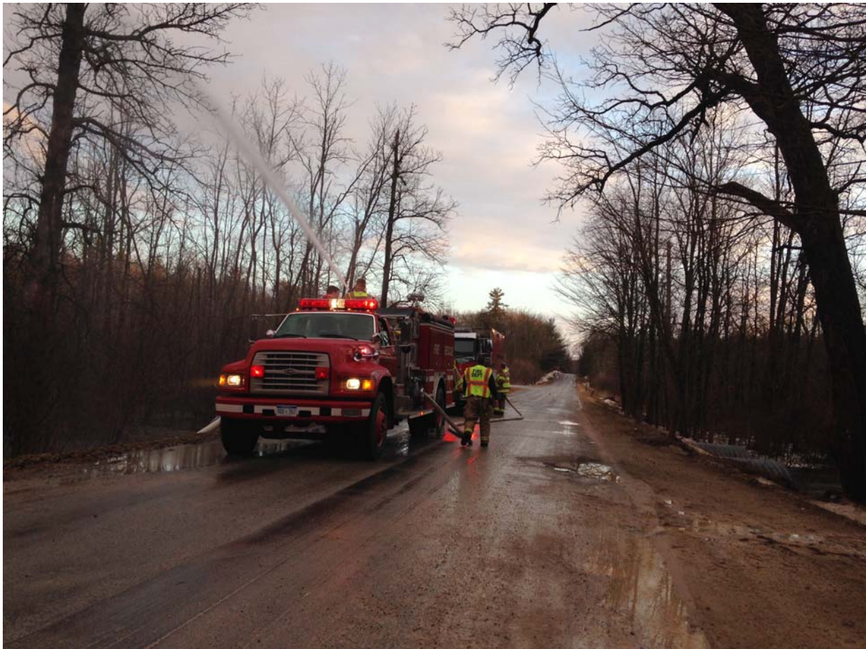
E-2 drafting water from Duke Creek dry hydrant on Division
